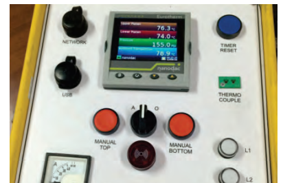
Electronic control box with data logger for regulating temperature
